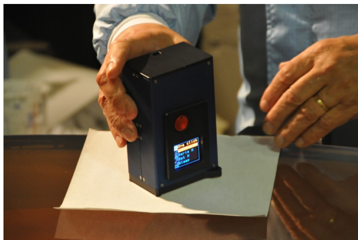
Taking a measurement with mirror protecting tissue.
