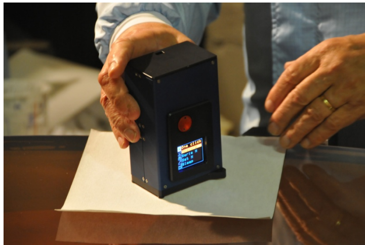
Taking a measurement with mirror protected by lint-free wiper.
