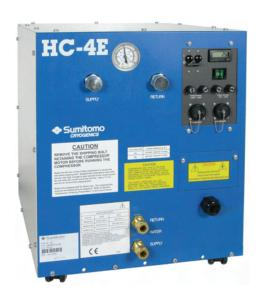
SHI Cryogenics Group's HC-4E1 compressor is designed to operate the Marathon® CP-8, CP-8LP and CP-250LP cryopumps along with a range of 10K cryocoolers. The compressor utilizes a water-cooled rotary compressor capsule designed exclusively to deliver high pressure, oil-free helium to cryogenic refrigerators. It is a reliable and compact system for both vacuum and laboratory operations, and like all Sumitomo Cryogenics products, is supported by a worldwide sales and service center network.
