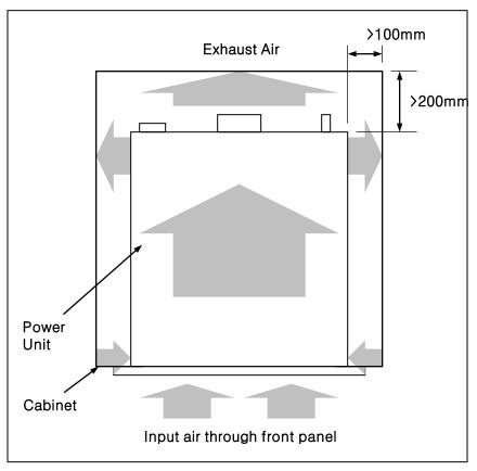
(Side clearance for the power unit in a cabinet)
